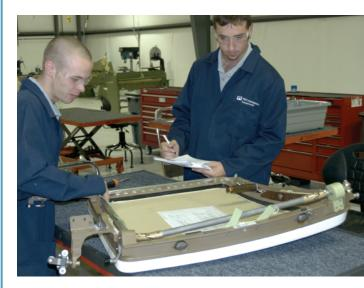
Above: Certified technicians inspect an overhauled Boeing 777 No. 2 framed window assembly.
