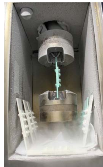
Testing of PR-2870 demonstrates outstanding corrosion protection.
