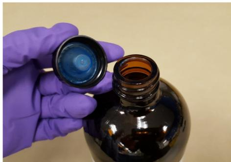
Open the container and ensure there is no crust or debris around the lid, and no FOD or particles in the container. The adhesion promoter should be a uniform liquid. If there are any particles and crystallization in the liquid, or any other signs of contamination, the container should be discarded.
