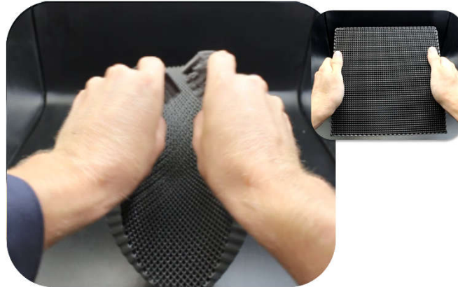
PPG ARE printed large elastomeric lattice
