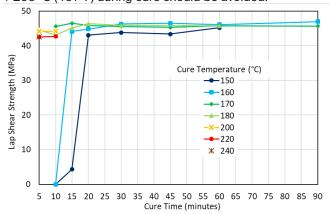
**Figure 2.** Range of cure times and temperatures that can be used to achieve optimum adhesive lap shear performance. All data collected using single lap joints prepared in the manner described below. Cure times and temperatures are that of the oven rather than that measured within the adhesive bondline.
