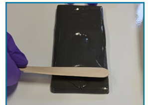
Sealant application & consistent layer (Buttering)
